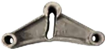
**Equalizer inspection is limited to three connection ports. The unit at left was caught just before catastrophic failure.**
